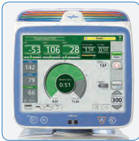
15 inch flat touch screen with wide viewing angle. 4 colored status display on top of the screen visible from any angle.
