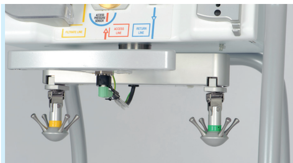
Scales The Aquarius system automatically compensates for ultrafiltration (UF) variations thanks to the scales.
