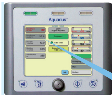
Renal Dose Displayed on the main screen in ml/kg/h so the user is fully aware of the dose of treatment achieved.
